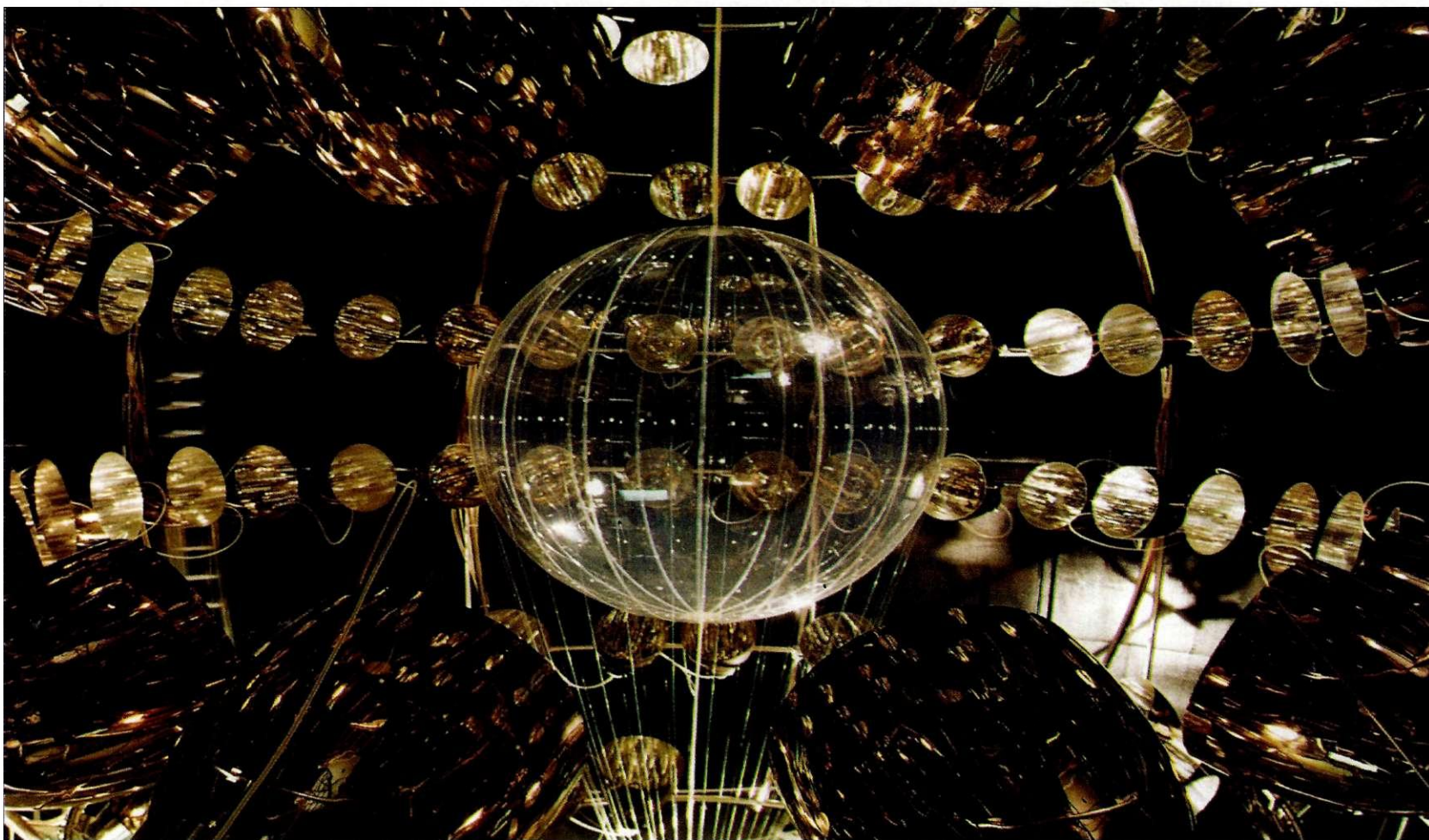
Fig. 2: The CTF is a scaled-down version of Borexino, with a nylon inner vessel containing 4.5 m 3 of scintillator. This shows a detail of the detector within the water tank, with the nylon inner vessel, some phototubes and optical concentrators visible.
